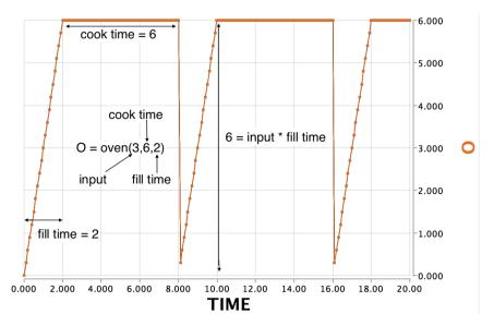
An oven exists in one of four states at any given time: idle, filling, cooking, or emptying. Initially, an oven is in the idle state. While idle, the oven watches its input for nonzero values. The oven will remain in this state indefinitely as long as its input remains zero. When the oven detects a change in the input, it adds that value to its contents and switches to the filling state.
